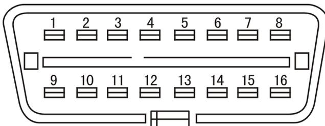
(2) With a numerical analysis and data transmission function(DATA LINK CONNECTOR-DLC).
